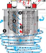
The three filters are protected by a special patented cyclone effect that prevents the problem of rapid filter clogging.
